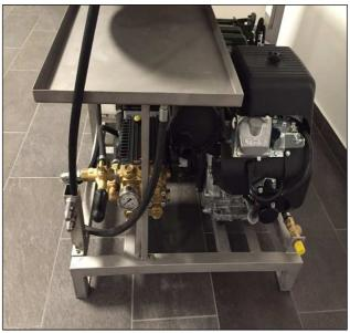
This unit is ideal for cleaning sewer pipes, drainage, flushing and cleaning before camera inspection. The special nozzle guarantees strong forward drive through the pipe.
