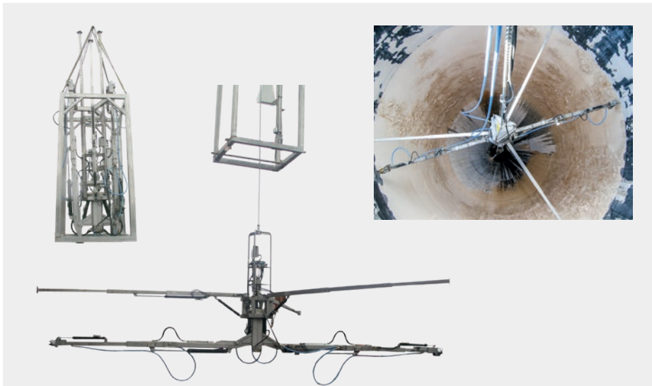
Cleaning system for very large vessels The system is designed for cleaning vessels up to 20 m in diameter. It is lowered into the vessel and fixed in position by three extendable support arms. The workarms with hydraulically driven rotor nozzles turn in a horizontal plane by means of a turntable, extend or retract hydraulically and swivel vertically powered by hydraulic cylinders.
