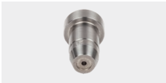
TYPE: L ROUND JET Op. pressure: up to 1200 bar Efficiency factor: 0.95 Material: Steel Nozzles: 1.0 – 3.9 mm
