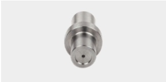
TYPE: A ROUND JET Op. pressure: up to 2000 bar Efficiency factor: 0.95 Material: Steel Nozzle: 0.4 – 4.9 mm
