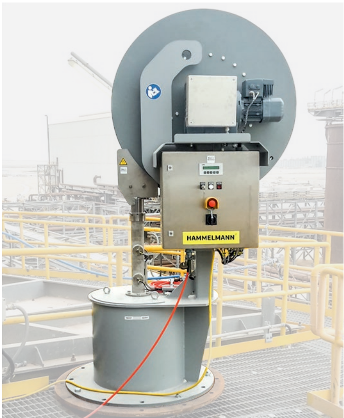
Hose reel system
