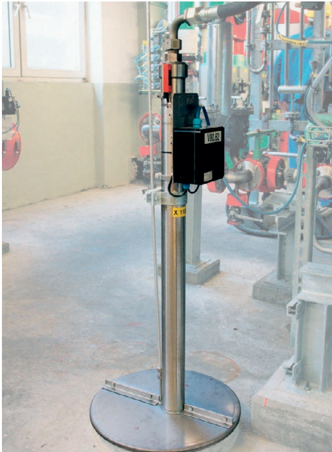
Lance system - moved hydraulically/pneumatically actuated
