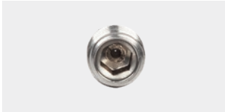
TYPE: G ROUND JET Op. pressure: up to 2500 bar Efficiency factor: 0.92 Material: Steel Nozzles: 0.25 – 1.2 mm
