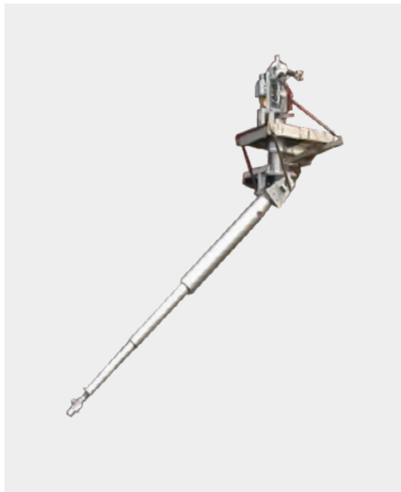
Swivellable telescopic cylinder The four-stage telescopic cylinder can be turned up to 180 degrees, swivelled 90° max. and can be extended up to 4 metres.
