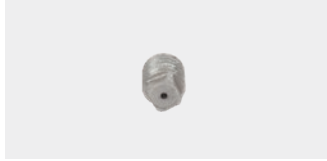
TYPE: S ROUND JET Op. pressure: up to 3000 bar Efficiency factor: 0.95 Material: Steel Nozzles: 1.0 – 1.8 mm
