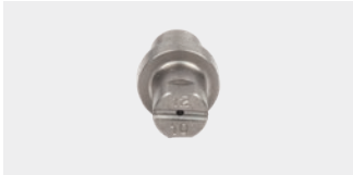
TYPE: B FAN JET Op. pressure: up to 2000 bar Efficiency factor: 0.67 Material: Steel Nozzles: 0.8 – 3.0 mm
