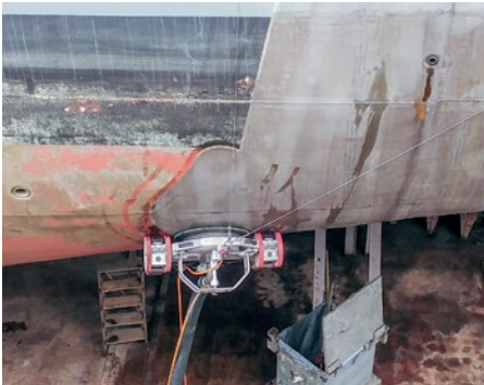
The Spiderjet V is held on the work surface by a vacuum, which at the same time suctions off the removed waste material and waste water.
