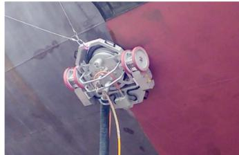
Spiderjet M - magnetically adhering surface cleaning device
