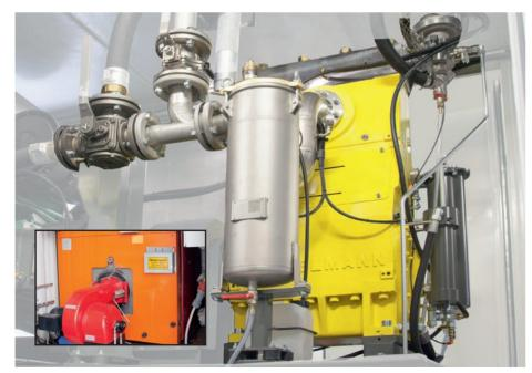
A separate water heating unit supplies hot water at boost pressure. High pressure is generated by the high pressure pump.
