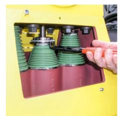
The vertical configuration of the Hammelmann pumps allows maintenance at typical working heights.
