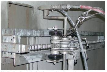
Mobile abrasive cutting injectors and handling equipment
