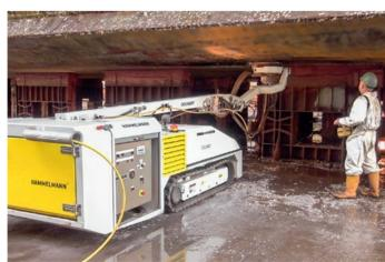
Dockboy - surface preparation on ship hull bottoms
