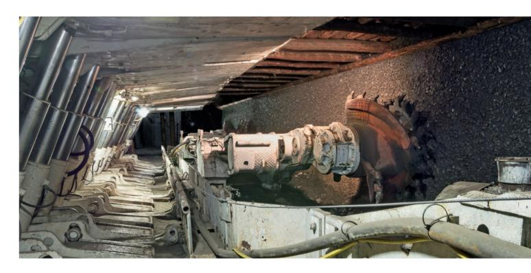
Special Hammelmann high pressure pump units for use underground have a base frame with high torsional rigidity. The filters and control elements have firedamp protection. The valve technology is designed for use in mining applications.
