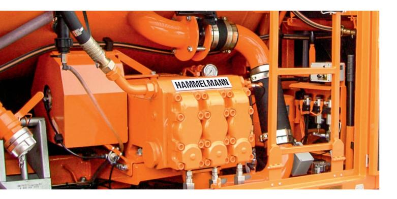
High pressure pumps with high flow rates suitable for use in recycling systems. The plungers are made of ceramic. A hermetic piston rod seal using bellows prevents oil leakage.
