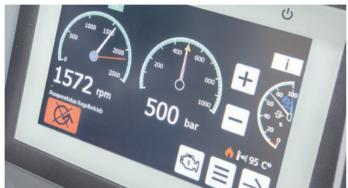
The heater module and the HDP 32 combined can produce an operating pressure of up to 500 bar reaching up to 95 °C of water temperature.
