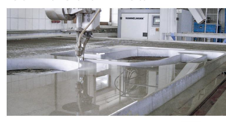
Hammelmann pumps make especially economic use of the energy utilized. Intelligent design, the use of high strength materials and precise manufacturing of components ensure long service life at pressures up to 4000 bar.
