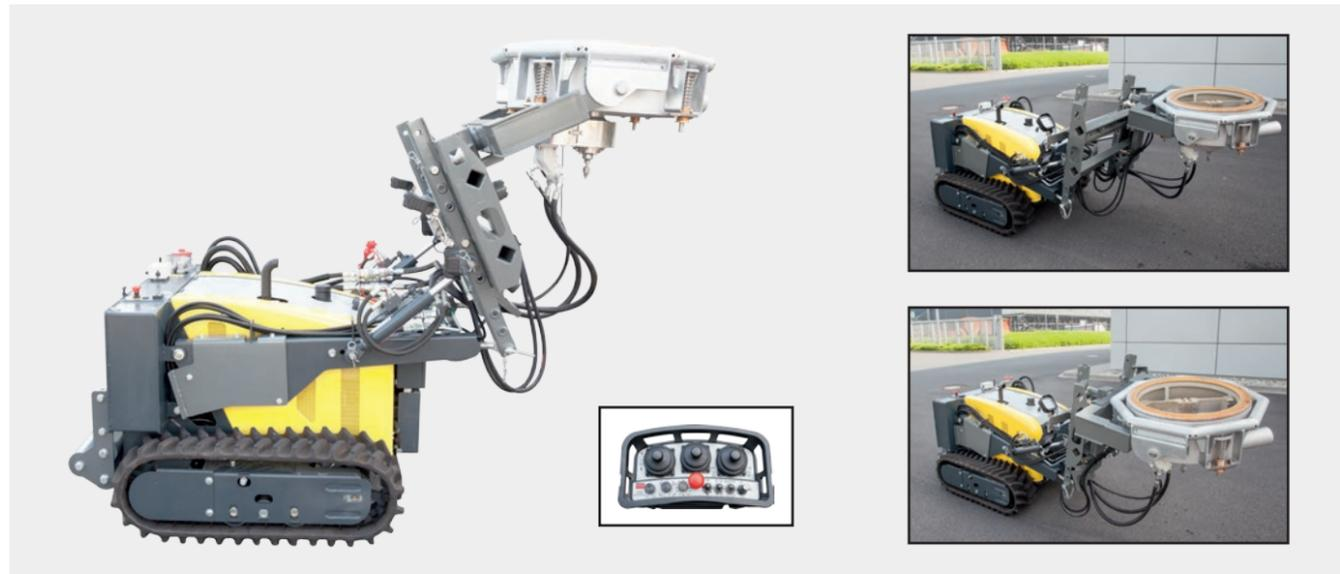
Self-sufficient carrier vehicle that can connect various jetting tools for surface treatment i.e. the cleaning and de-coating of ship decks,
